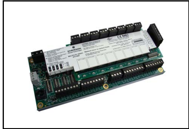
Figure 2-4 - RoHS MultiFlex Combination Input/Output Board (Side View)
