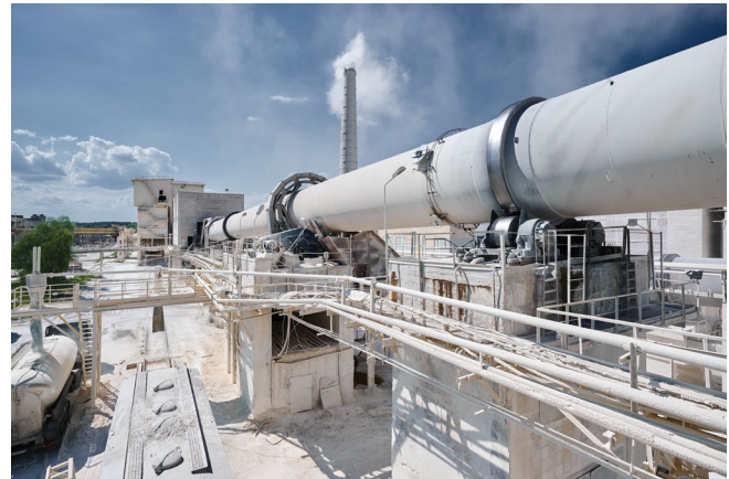
Figure 4: Rotary kilns have a wide range of efficiency ratings, often related to age.
