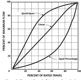
Figure 2. Flow vs. Travel of Various Cage Styles
