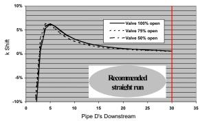
Figure 5: Butterfly Valve Errors 90° Off Valve Axis
