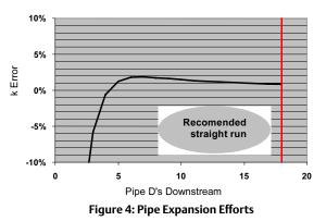
485 Annubar Butterfly Valve Errors Annubar Oriented 90° off Valve Axis
