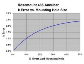
Figure 1: K Error vs. Mounting Hole Size
