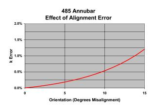
Figure 2: Effect of Alignment Error
