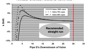
Figure 6: Butterfly Valve Errors Parallel to Valve Axis
