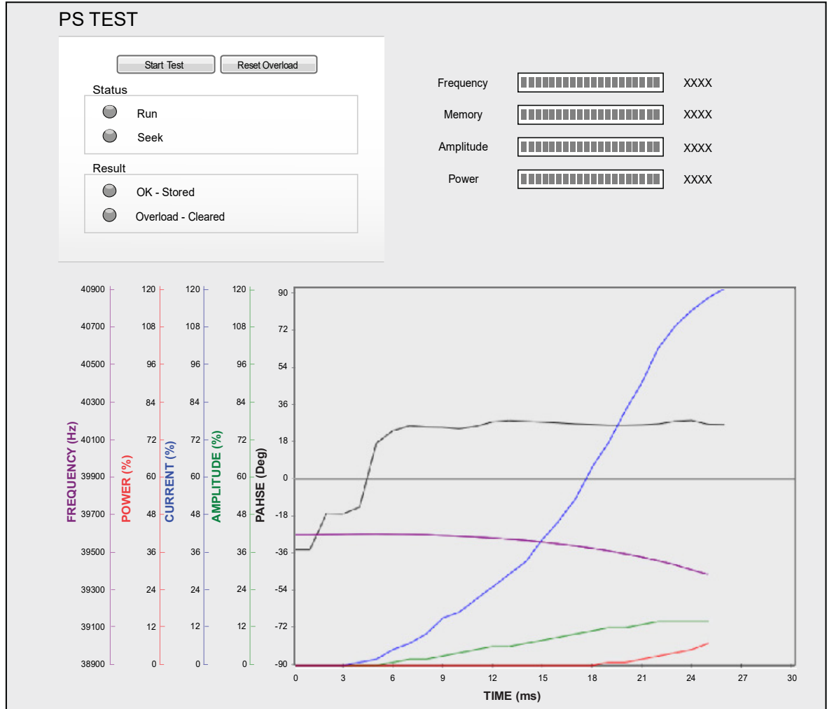
Figure A.11 Weld Graph, Defective Converter
