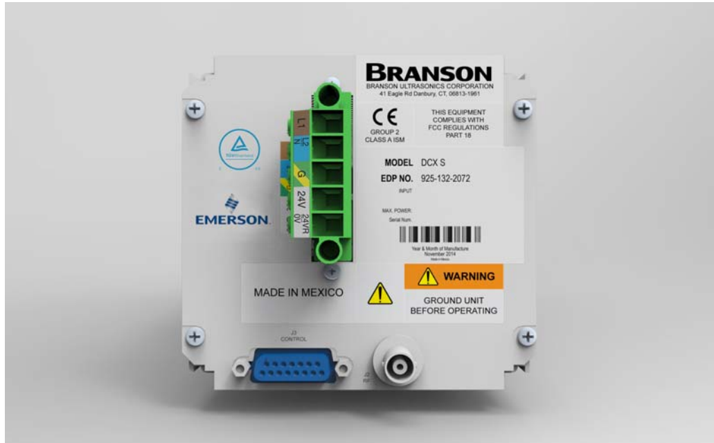
Figure 1.2 Safety-related Labels found on the DCX S Power Supply
