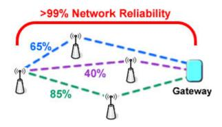
A self-organizing network – even with path reliabilities of less than 99% – can still create reliable paths for communication.
