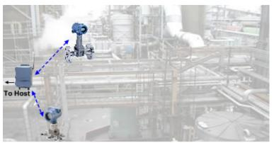
In the simplest configuration of a self-organizing network, wireless devices communicate directly with the gateway.
