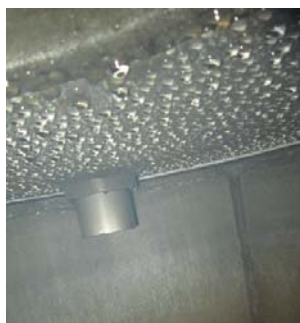
Figure 7. The End of the 2-in Rosemount 5408 Antenna
