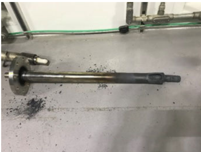
Figure 4: Severe Heat Degradation and Embrittlement at Nozzle End
