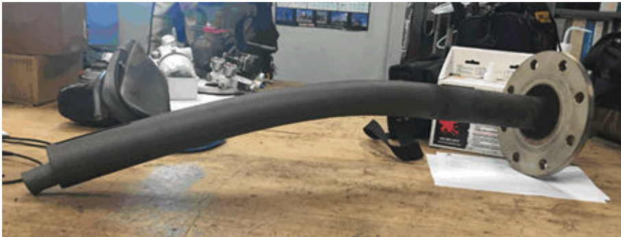
Figure 6: Thermal Creep Causing a Sag of 2 inches per ft
