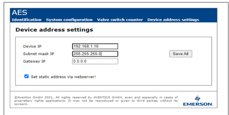
Fig. 14: Example of IP address with web server
