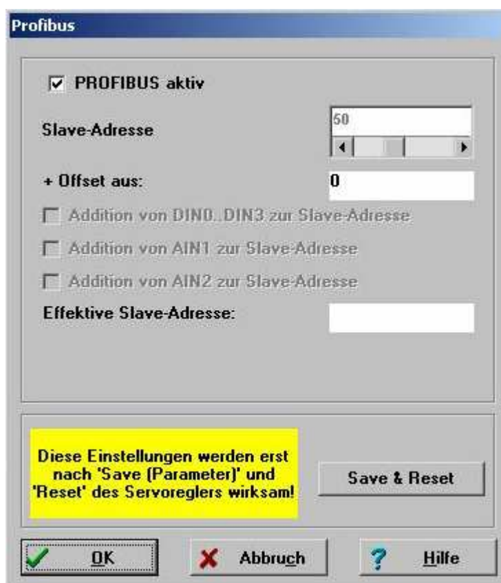
Figure 7.1: Setting the operating parameters
