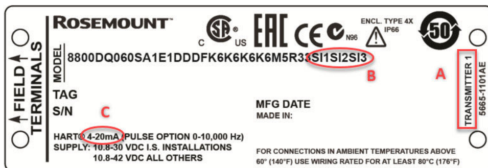
Figure 2-2: Example of Quad transmitter nameplate
