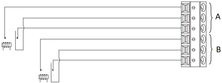
Figure 2-3: Alarm indicator relay terminals
