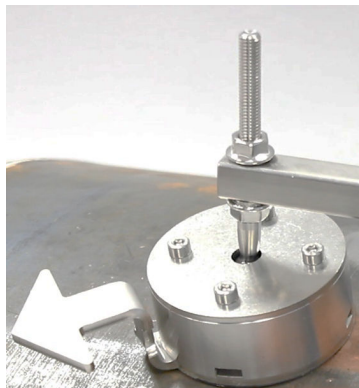
Figure 5-6: Fitted Protective Cap
