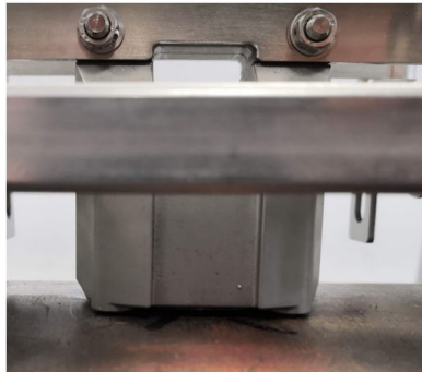
Figure 4-10: ET410 in Contact with Vessel inside Magnetic Fixture
