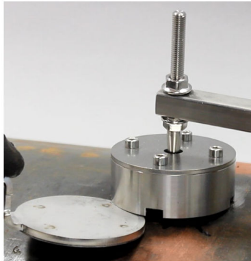
Figure 5-5: Refitting the Protective Cap
