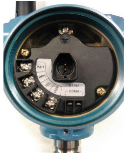
Figure 2-1: Terminal Wire Colors
