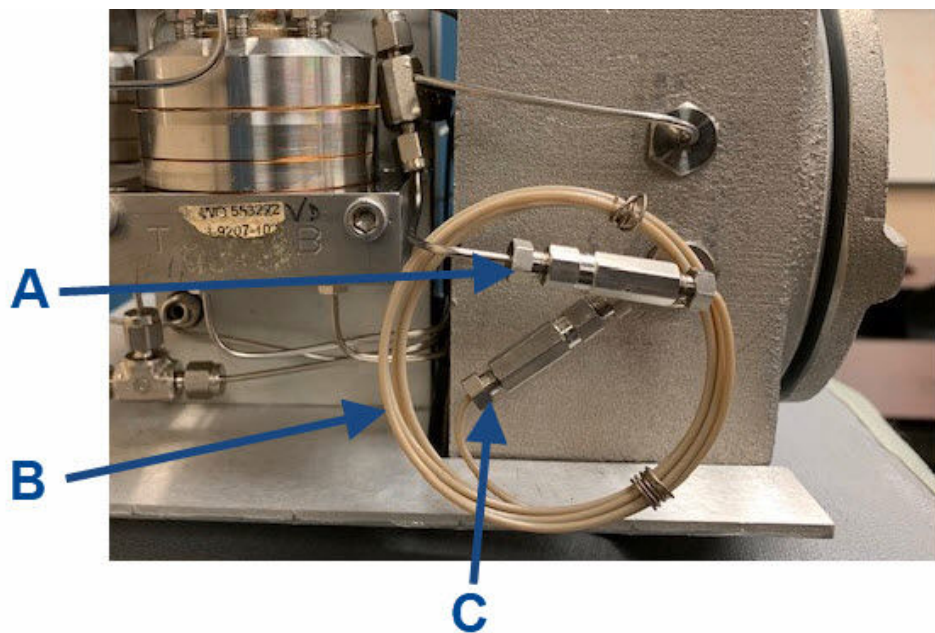
Figure 2-3: New 10-ft. (3 m) Restrictor (R2)
