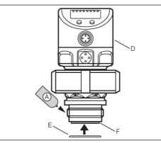
The adapter comes with an EPDM O-ring. More sealing rings are available. For more information see the transmitter datasheet or visit Emerson.com/Rosemount.
