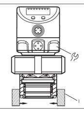
8. Tighten the transmitter to a torque of 25.81 ft/lbs (35 Nm).
