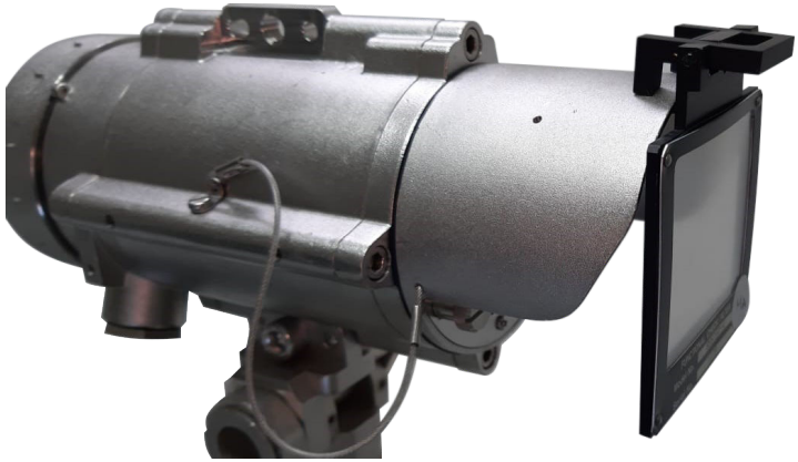
Figure 2-5: Receiver with Check Filter Installed
