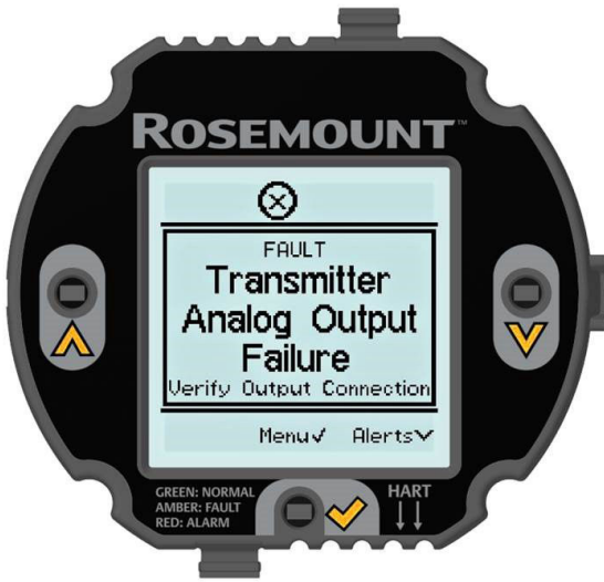
Figure 2-15: Current Loop Fault Screen
