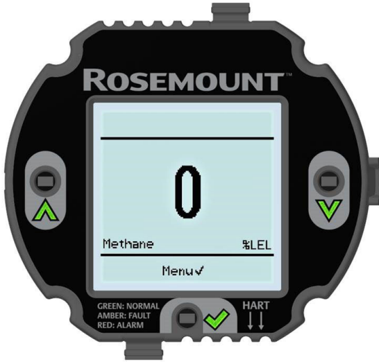
Figure 2-14: Primary Variable Screen Using Methane
