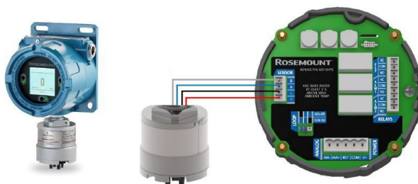
Figure 2-7: Remote mount wiring diagram: 905 to 925
