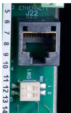
Figure 3-12: SW1 switches on the backplane
