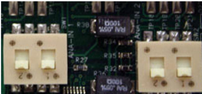
Figure 3-27: Factory settings for analog input switches
