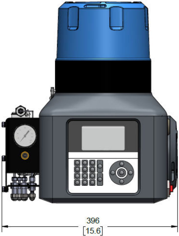
Figure 2-3: 470XA dimensions collapsed
