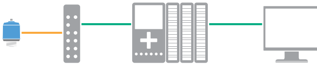
Figure 5-3: Connection via the PLC
