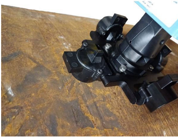
Figure 2-8: First magnet housing attachment
