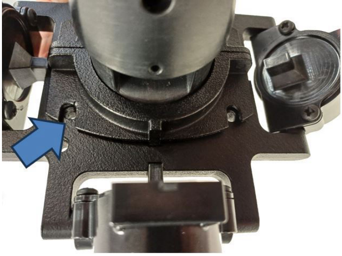
Figure 2-4: Ensuring alignment of Transmitter in vessel mount frame
