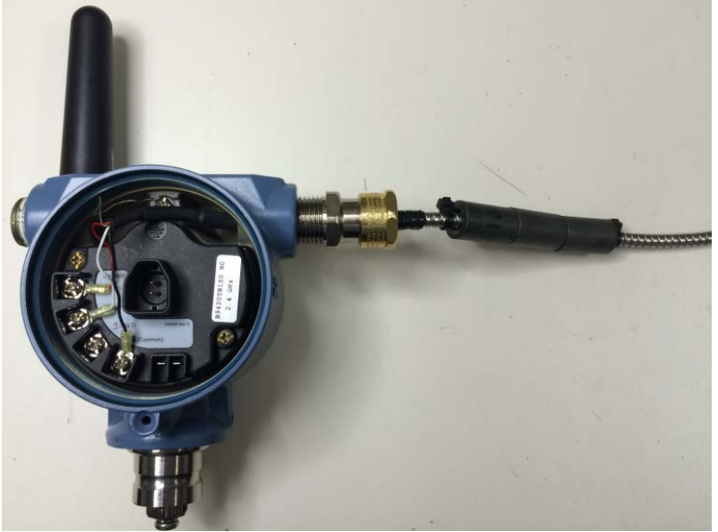
Figure 5-2: AMS 9420 with armor-jacketed cable and ferrites
