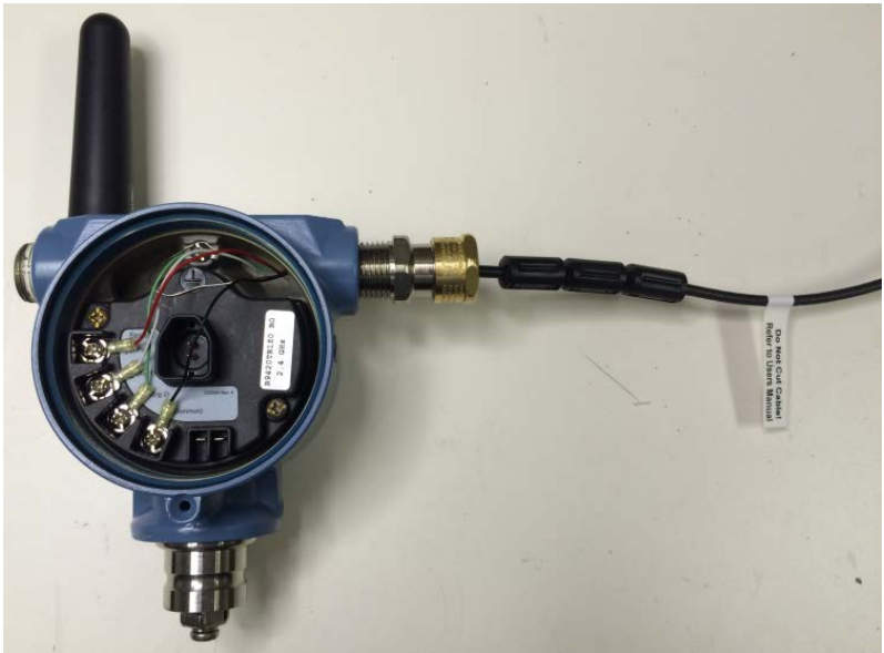
Figure 5-1: AMS 9420 with standard cable and ferrites
