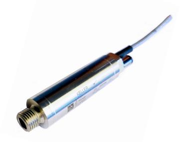
The VPS 58, Vapor Pressure Sensor, is installed as an integrated part of the Tank Radar Gauge. The intrinsically safe sensor is installed with the purpose of measuring the vapor pressure and provide the relative pressure inside the cargo tank. The signals from the sensor are processed by the tank gauge electronics and transmitted to the Supply and Communication Unit over the same interface as the radar and temperature signals.
