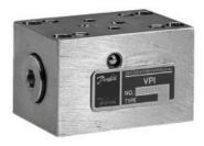
Pressure and temperature compensating block primarily for analog indication (VPI-C). The PTC-Block allows the compression/ decompression of the oil in the system caused by major temperature and pressure variations, without influencing the indicator, and ensures precise intermediate positions, as the positioning is always made at constant pressure (5 bar). The PTC-Block is provided with CETOP-3 connection for mounting of solenoid pilot valve.
