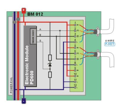
Please note that the 4-Wire P-NET screen has to be terminated /connected to the ground of the panel.
