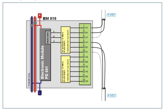
The BM 010 base module is equipped with termination circuits for the two P-NET channels. It is recommended to enable the termination circuit when the device is installed at the terminal ends of a transmission cable. Enabling/disabling the termination circuit is done via jumper settings.
