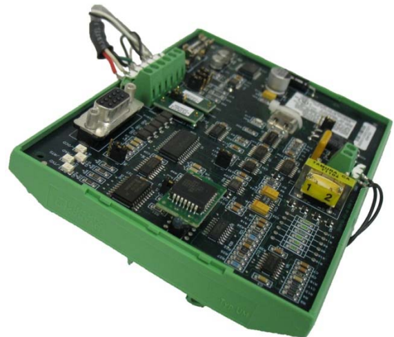
ControlWave HART Device
