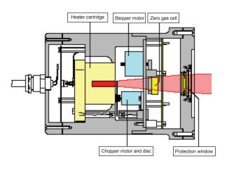
Model 5500 Analyzer Transmitter
