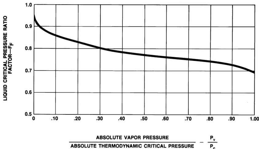
USE THIS CURVE FOR LIQUIDS OTHER THAN WATER. DETERMINE THE VAPOR PRESSURE/CRITICAL PRESSURE RATIO BY DIVIDING THE LIQUID VAPOR PRESSURE AT THE VALVE INLET BY THE CRITICAL PRESSURE OF THE LIQUID. ENTER ON THE ABCISSA AT THE RATIO JUST CALCULATED AND PROCEED VERTICALLY TO INTERSECT THE CURVE. MOVE HORIZONTALLY TO THE LEFT AND READ THE CRITICAL PRESSURE RATIO,  $F_p$ , ON THE ORDINATE.
