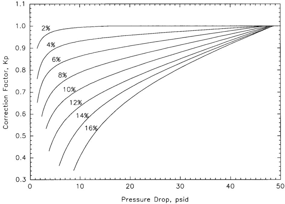
Figure 2. Pulp Stock Correction Factors for Mechanical Pulp
