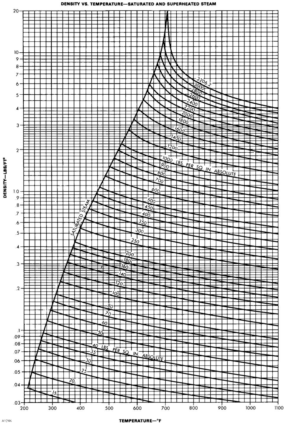
The degree of superheat is the difference between the actual temperature and the saturation steam temperature.
