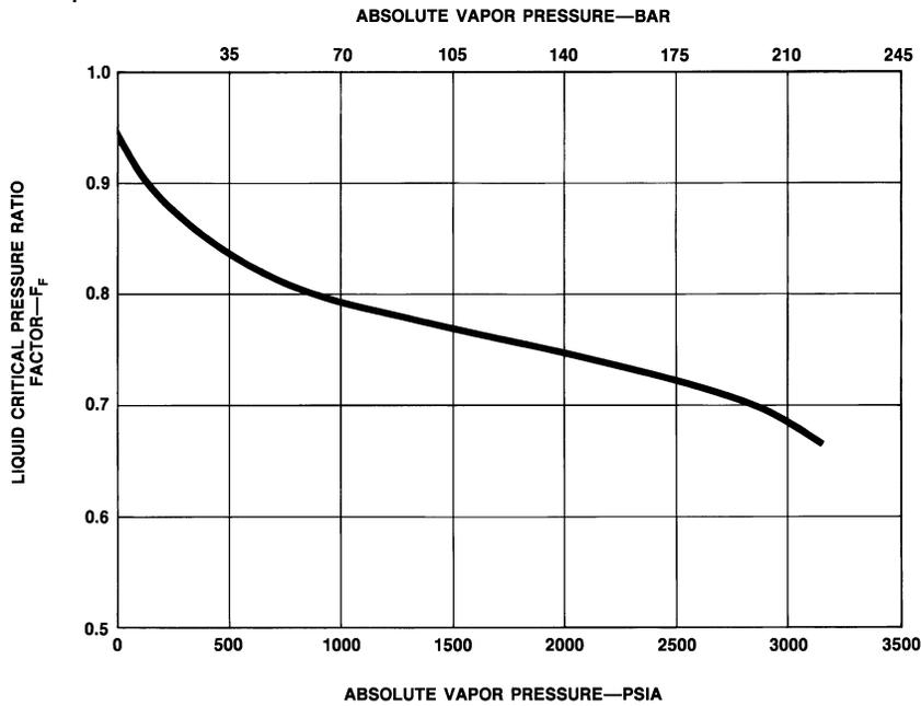
USE THIS CURVE FOR WATER. ENTER ON THE ABCISSA AT THE WATER VAPOR PRESSURE AT THE VALVE INLET. PROCEED VERTICALLY TO INTERSECT THE CURVE. MOVE HORIZONTALLY TO THE LEFT TO READ THE CRITICAL PRESSURE RATIO,  $F_p$ , ON THE ORDINATE.
