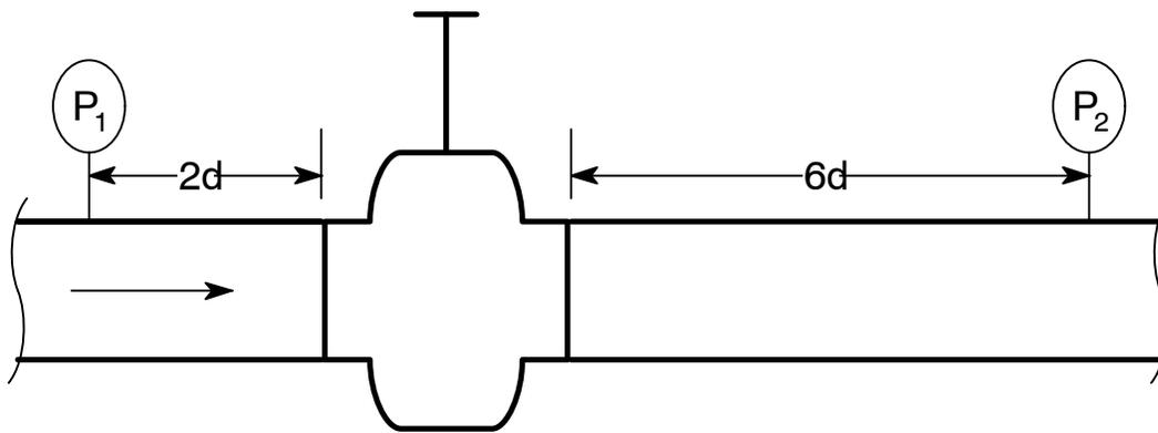
The control volume as defined by ISA 75.01.01 includes two diameters of piping upstream of the valve and six diameters downstream. This allows the fluid to fully develop prior to entry into the valve and enough time to recover downstream of the valve when  $C_V/d^2 \leq 30$ . For these cases where  $C_V/d^2 > 30$ , alternative methods need to be considered.
