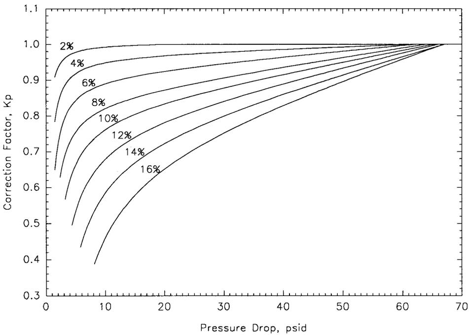
Figure 3. Pulp Stock Correction Factors for Recycled Pulp
