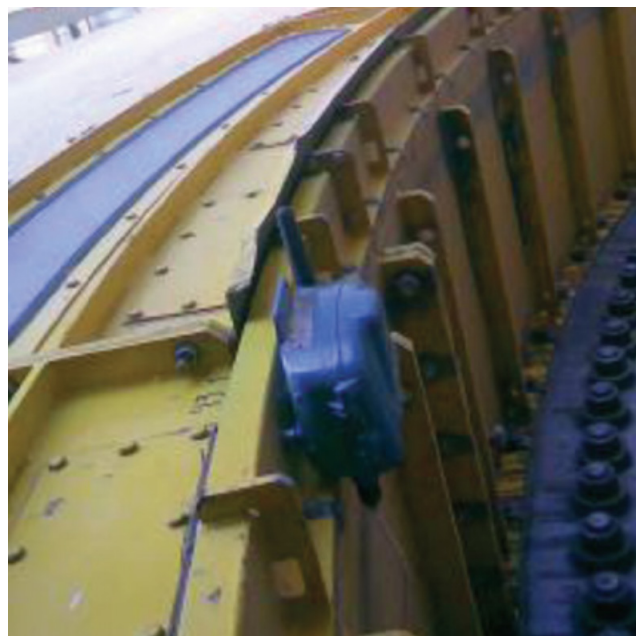
Figure 3. The Rosemount 848T High Density Wireless Transmitter accepts up to four independently configurable inputs, dramatically reducing installation and operational costs per point through the use of a smart, reliable, and secure wireless network.
