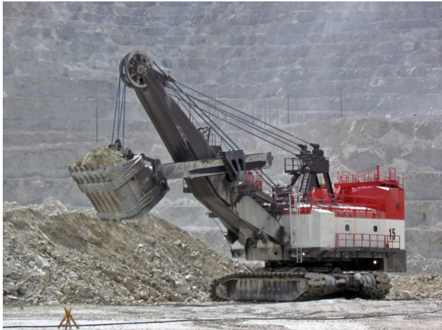
Figure 1. It is vital to monitor the condition of key electric rope shovel components – the crowd, hoist, and swing drives – all of which are vulnerable to failure.
