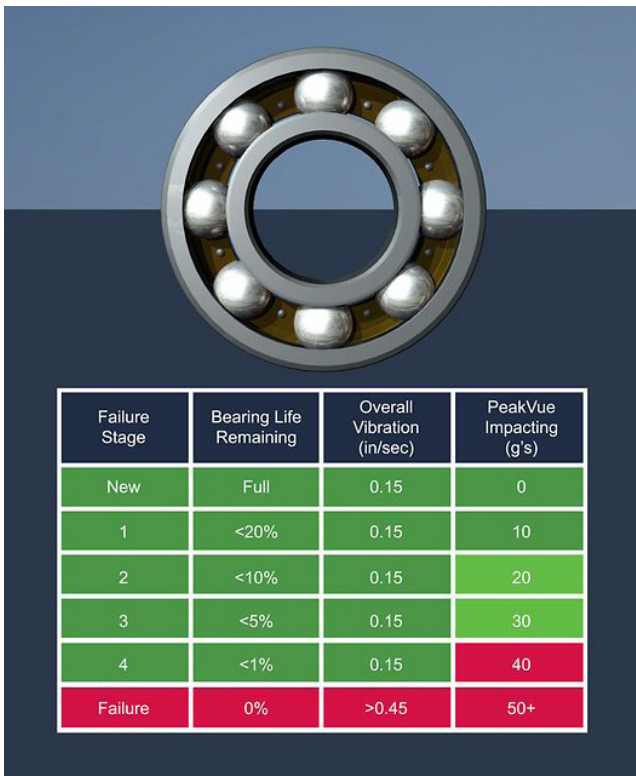
Figure 2. Peak value analysis technology, such as PeakVue from Emerson, can deliver unprecedented insight into the operating condition of critical pit assets, to determine when rotating equipment is healthy, and when an abnormal situation is present.
