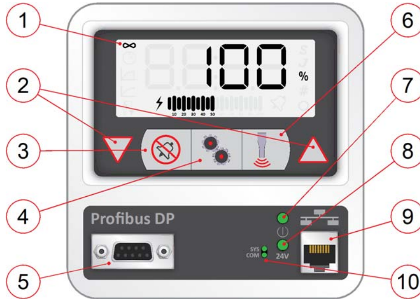
Figure 2.3 DCX F-DP Power Supply Front Panel Controls and Indicators
