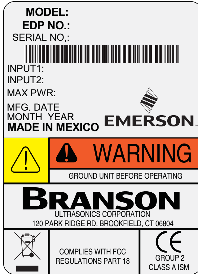
Figure 1.1 Safety-related Labels found on the DCX F-DP Power Supply
