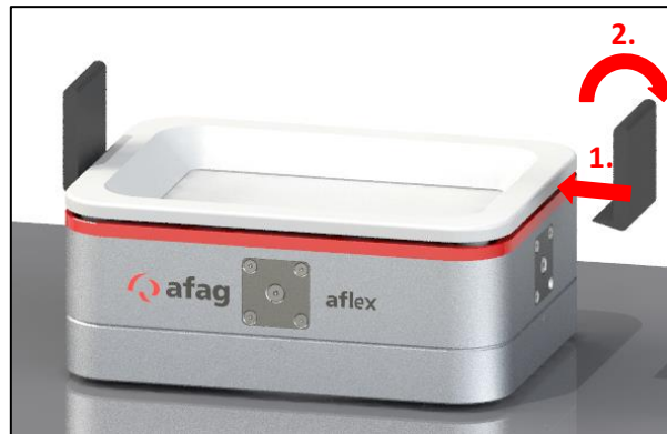
Figure 7: Motion sequence dismantling funnel plate with assembly wedges
