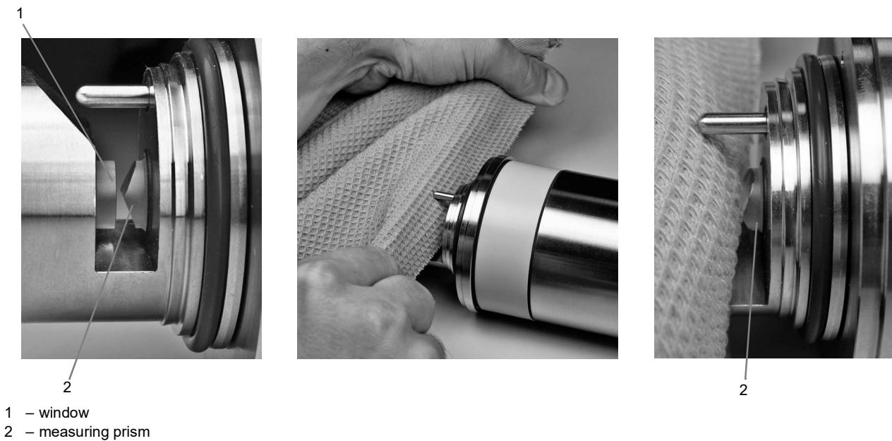
Fig. 11.1: Cleaning of measuring prism and window
