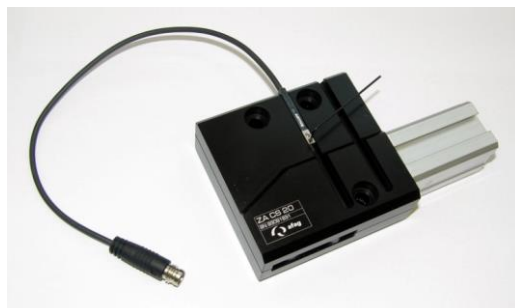
Fig. 21 Mounting the proximity switch in the ZA module
