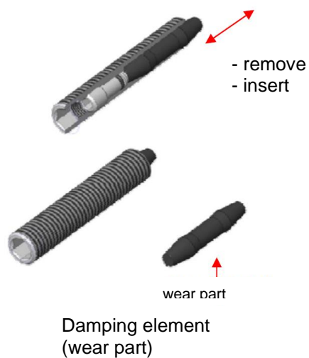
Fig. 26 Replacing the damping elements (elastomer shock absorbers)
