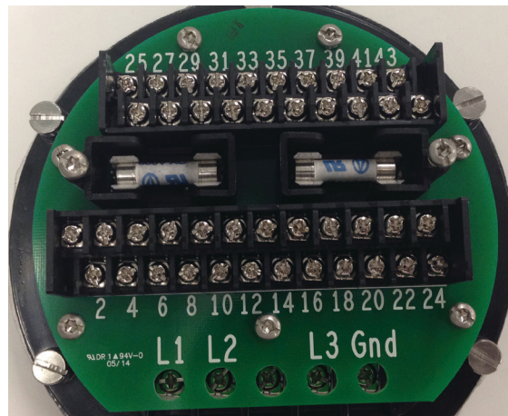
Figure 7-1 Fuses in the STC
