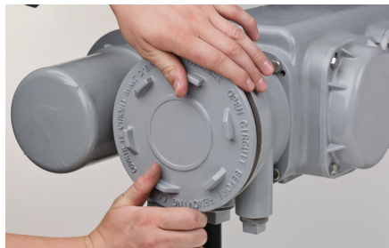
Figure 3-2 Removal of STC Cover
