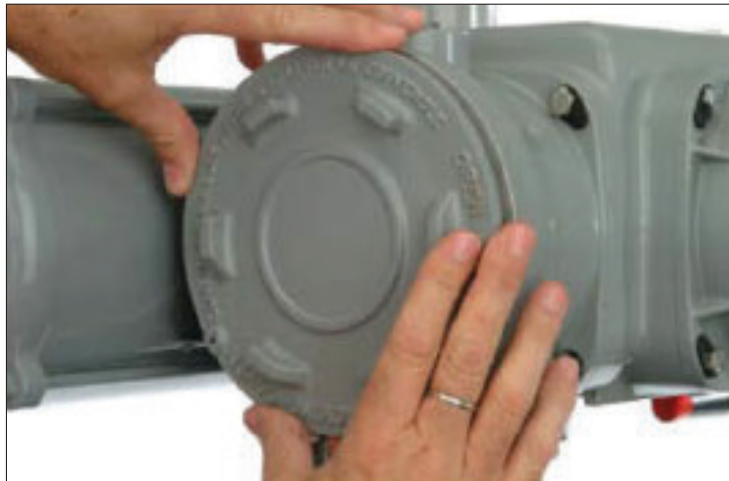
Figure 8 Remove STC Cover Turning Counterclockwise
