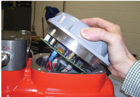
Figure 18 Remove Cover for Limit Switch Chamber
