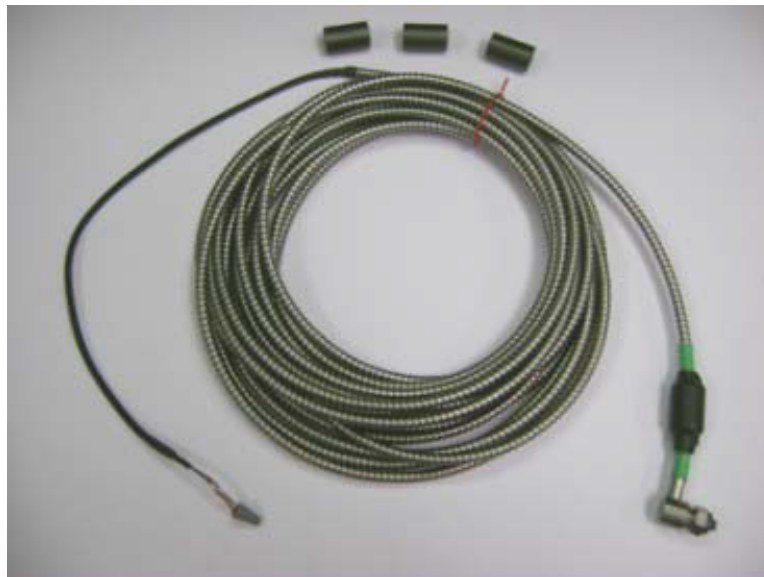
Figure 6-6: Armor-jacketed cable and ferrites (pre-installation)
