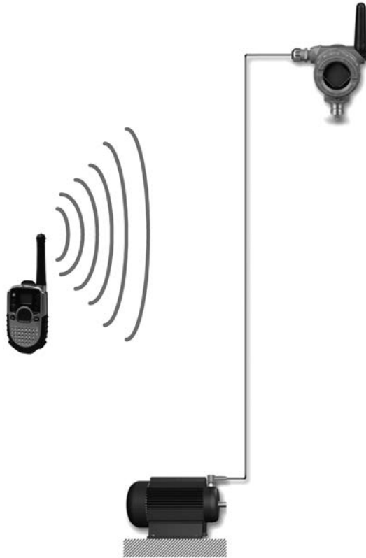
Figure 6-12: RFI source polarization coincident with long cable run (maximum interference)
