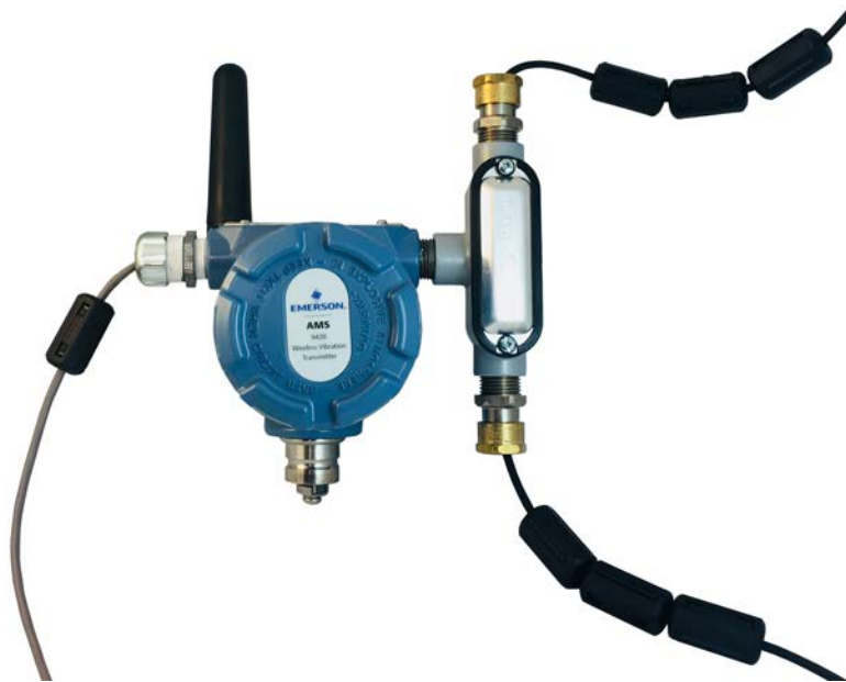
Figure 6-9: Ferrites installed on external DC supply and sensor cables
