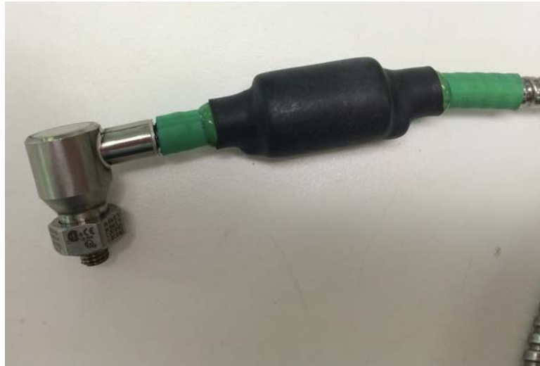
Figure 6-4: Armor-jacketed accelerometer cable with ferrite installed (as shipped from the factory)
