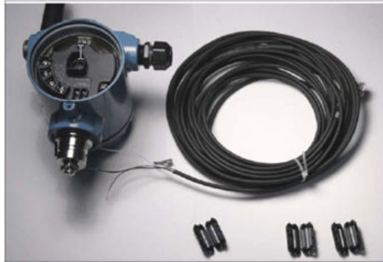
Figure 6-5: Transmitter, accelerometer with standard cable, and ferrites (pre-installation)
