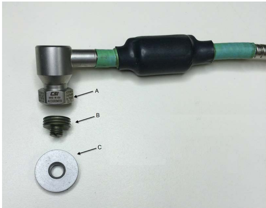
Figure 2-3: Accelerometer, mounting stud, and optional mounting pad
