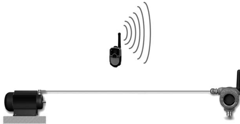
Figure 6-11: RFI source cross-polarized with long cable run (minimum interference)
