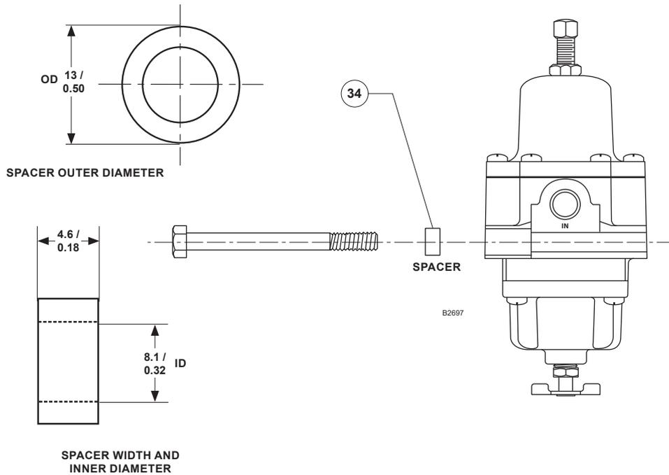
**Figure 1. Spacer Diameter and Assembly**
