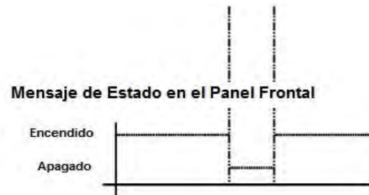
Fig. 5-3: Pre-alarma Alta y Alarma Principal
