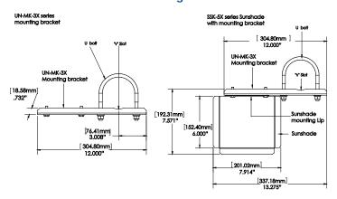
Figure 5 UNMK-3X with SSK-5X parts list
