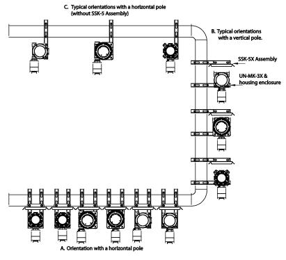
Figure 4 UNMK-3X & SSK-5X dimensional drawing
