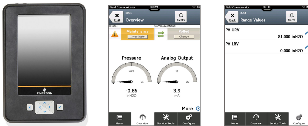
Figure 4-10: Before Zero Trim Using Field Communicator
