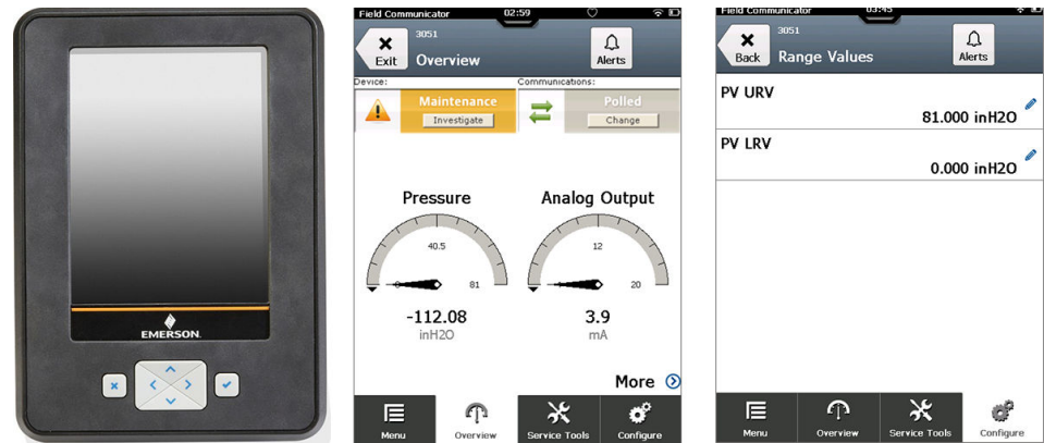
Figure 4-15: Before Re-range Using Field Communicator
