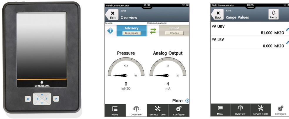
Figure 4-11: After Zero Trim Using Field Communicator
