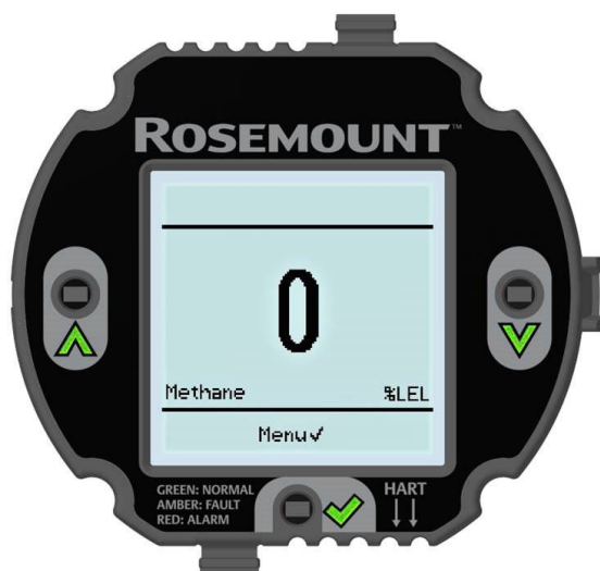
Figure 3-28: Primary Variable Screen Using Methane
