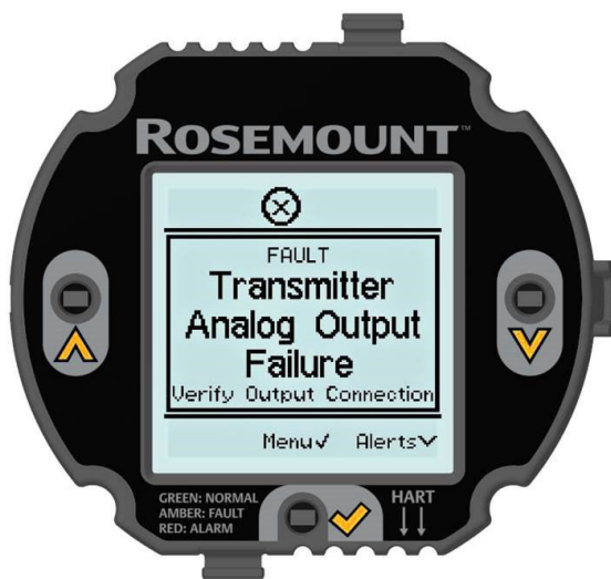
Figure 3-29: Current Loop Fault Screen
