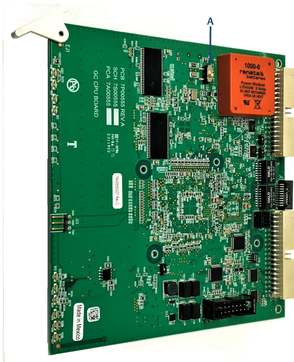
A. SW7 switch ( ON is towards the dot.)
