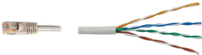
Figure 5-14: Crimped CAT5 cable
