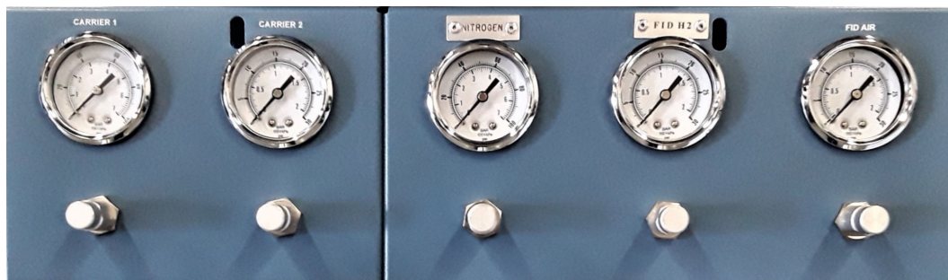
Figure 3-9: Regulators and gauges
