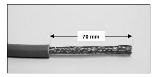
2. Cut and remove the metal braiding so that there is a minimum of 15 mm remaining.
