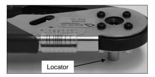
6. Insert the stranded wire into the crimp contact and then fully insert the crimp contact into the locator. Cycle the tool to create the crimp. Repeat this step for the remaining conductor wire(s).
