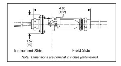
Figure 3-5 – Dimensional Drawing of Coupled Connector – Side Entry Hood Original Stainless Steel (Up to February 2020)
