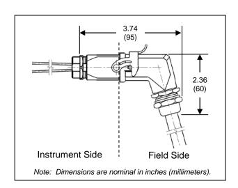
Figure 3-4 – Dimensional Drawing of Coupled Connector – Top Entry Hood Original Stainless Steel (Up to February 2020)
