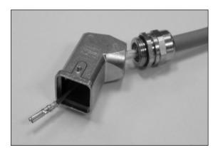
2. Making sure that the lead wires do not hang up on anything, screw the connector hood onto the cable gland as shown. Do not allow the conductor wires to become twisted.
