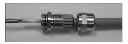
5. While using one of the 22 mm open-end wrenches to keep the metal base steady, screw the dome nut onto the metal base until finger tight. Then use the second 22 mm open-end wrench to tighten the dome nut an additional half turn. Ensure that the metal base is held steady during this entire step to prevent damage to the metal braiding on the cable.
