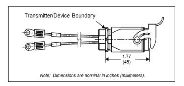
Figure 2-4 – Dimensional Drawing of Instrument Side, Stainless Steel
