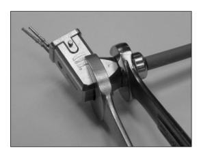
4. Check the instrument side connector to determine which pin (#1 or #2) is designated as the positive (+) pin. Insert the positive (+) field side contact into the correct pin location of the crimp terminal. Follow the same procedure for the negative (-) wire and the ground wire (if applicable). Consult the factory regarding 4-wire configurations.
