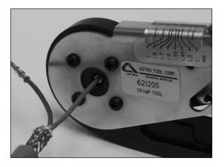
7. Properly installed crimp contact is shown in the following photo.
