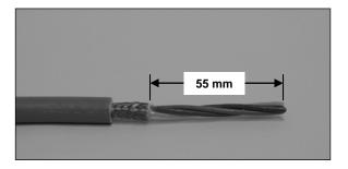
Cut any unused conductor wires flush with inner sheath. Strip 8 mm of insulation from the remaining wires, taking care not to cut or damage individual strands. Gently re-twist the stranded conductors if necessary.
