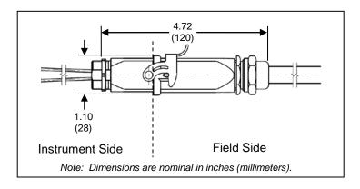
Figure 3-3 – Dimensional Drawing of Coupled Connector – Side Entry Hood
