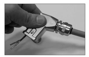
3. Using a 25 mm open-end wrench on the connector housing and a 22 mm open-end wrench on the cable gland, tighten the two pieces together. Then use an open-end torque wrench to tighten the cable gland to 22 ft-lb (30 N-m).
