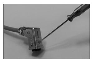
8. If the connector will not to be installed right away, attach the protective cap onto the connector hood.
