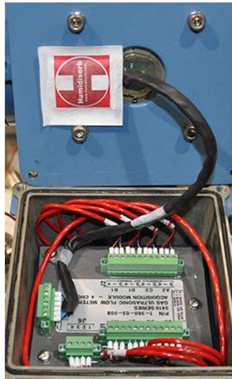
Figure 3-17: 3415, 3416, 3417 Ultrasonic Meter Acquisition Module wiring
