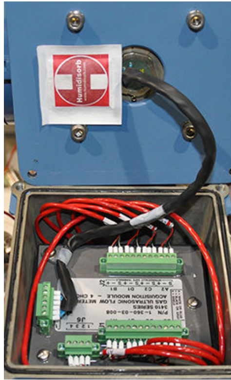
Figure 3-16: 3410 Ultrasonic Meter Acquisition Module Wiring
