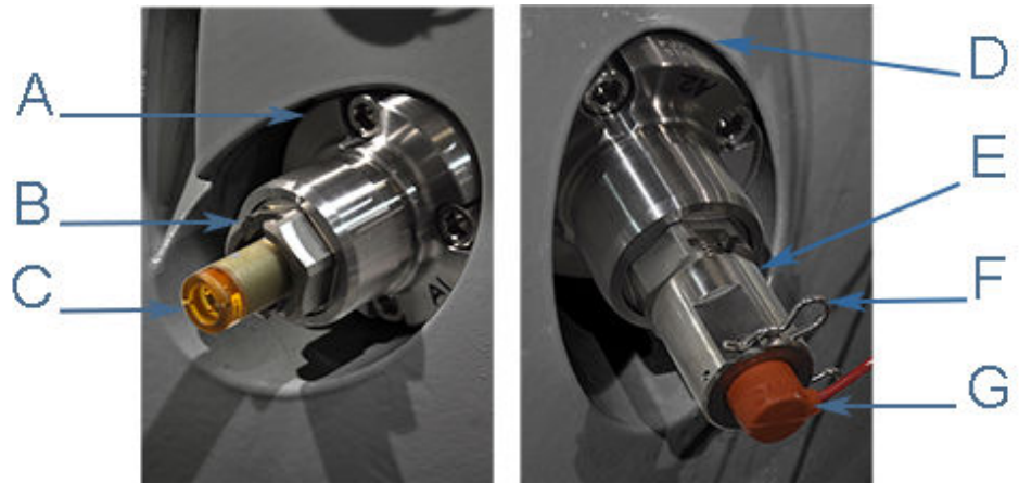
Figure 3-4: T-21 and T-22 transducer assembly, holder, transformer assembly, retainer, retaining clip, and transducer cable
