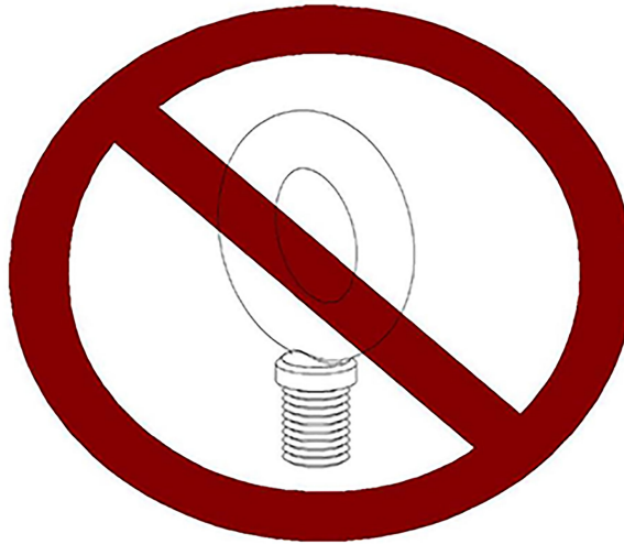
Figure 2-12: Non-compliant eye bolt
