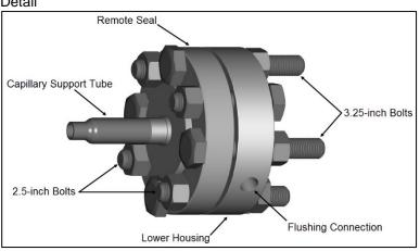
Figure 3-3 – Bolt Torqueing Pattern
