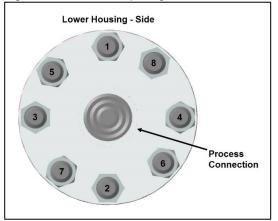
Figure 3-4 – Torqueing Pattern for Bolts Provided with Rosemount Spares Kit P/N 03159-5904-0003
