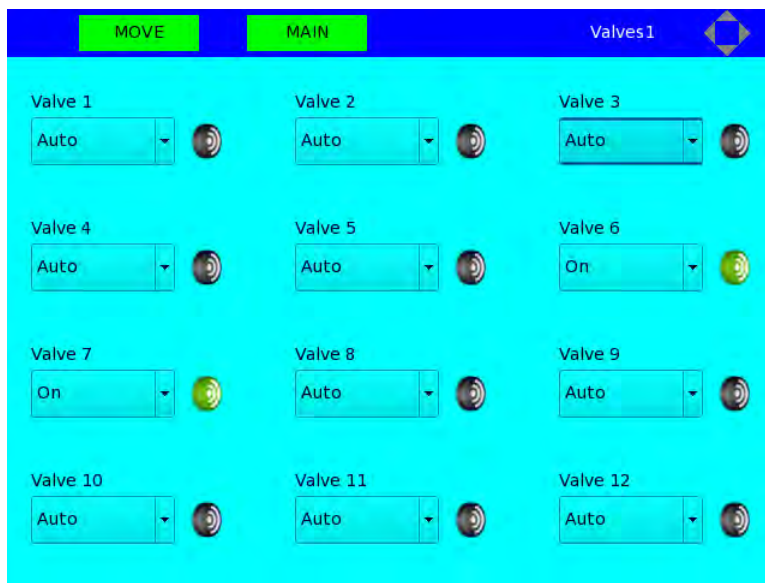
Figure B-28: Valves Screen
