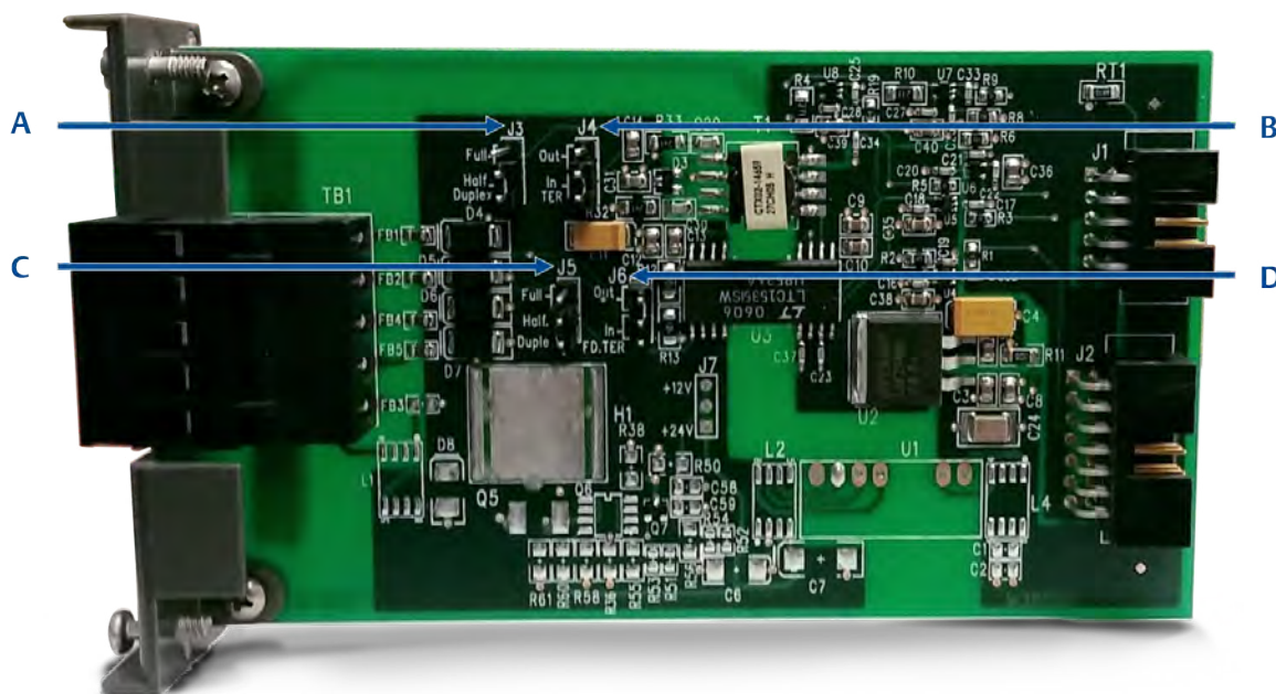
Figure 4-7: RS-485/RS-422 Jumper Settings on Serial Board
